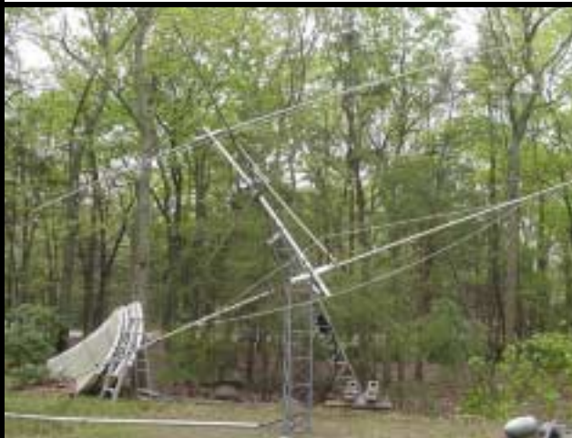
K2TXB is pointing at the moon with a pair of long yagis on a polar mount, polarization steering and using JT44
